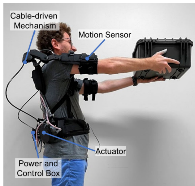
Fig. 1 Portable robotic exoskeleton for powered assistance during arms elevation. The robot detects residual volitional movements of the wearer’s limbs and provides support to offload the limbs from the effects of gravity, helping to restore arm functions in people with upper-limb impairments
